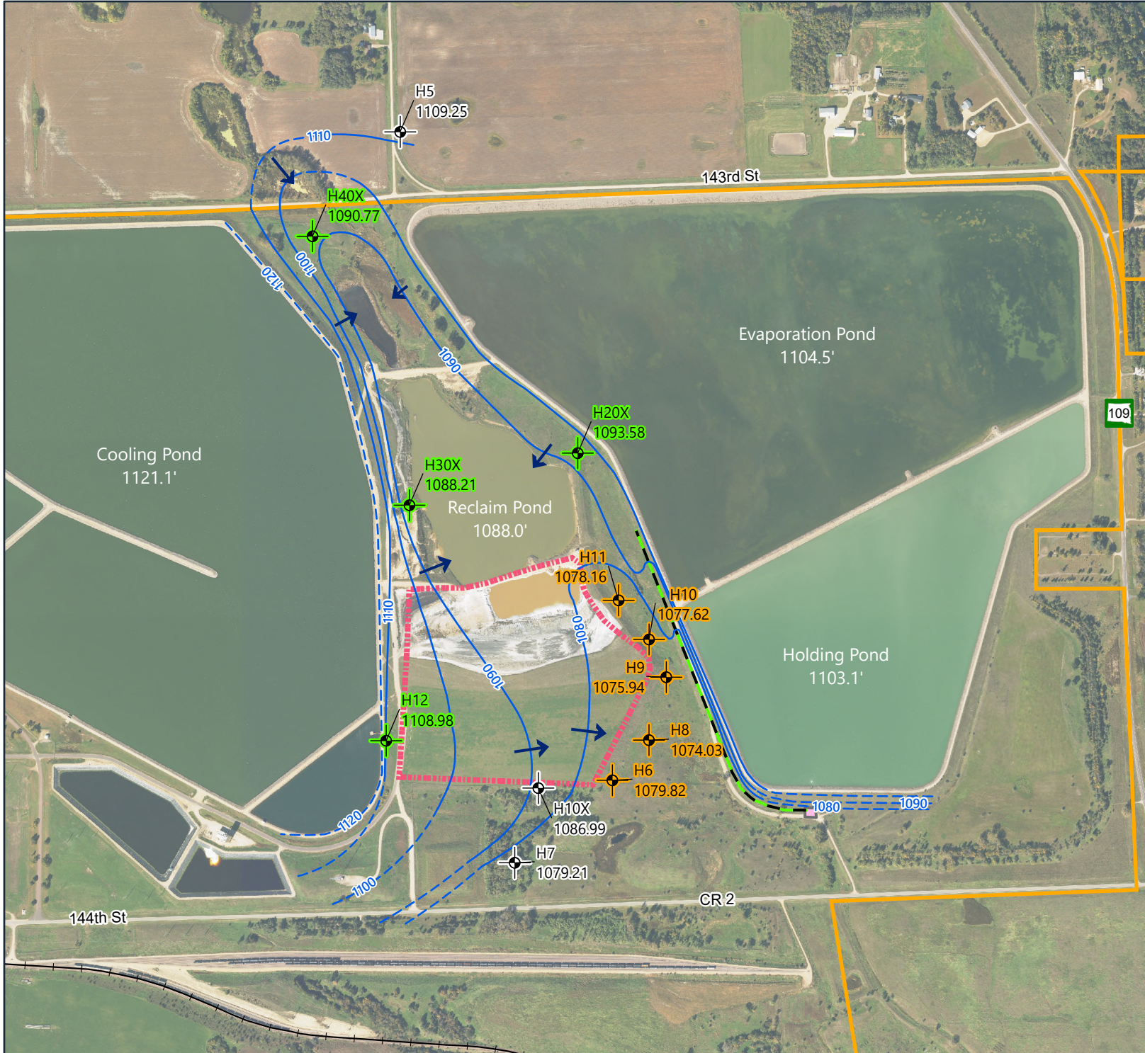
Groundwater Elevation Contours Spring 2025 Big Stone Plant Big Stone City, SD Otter Tail Power Company FIGURE 2
