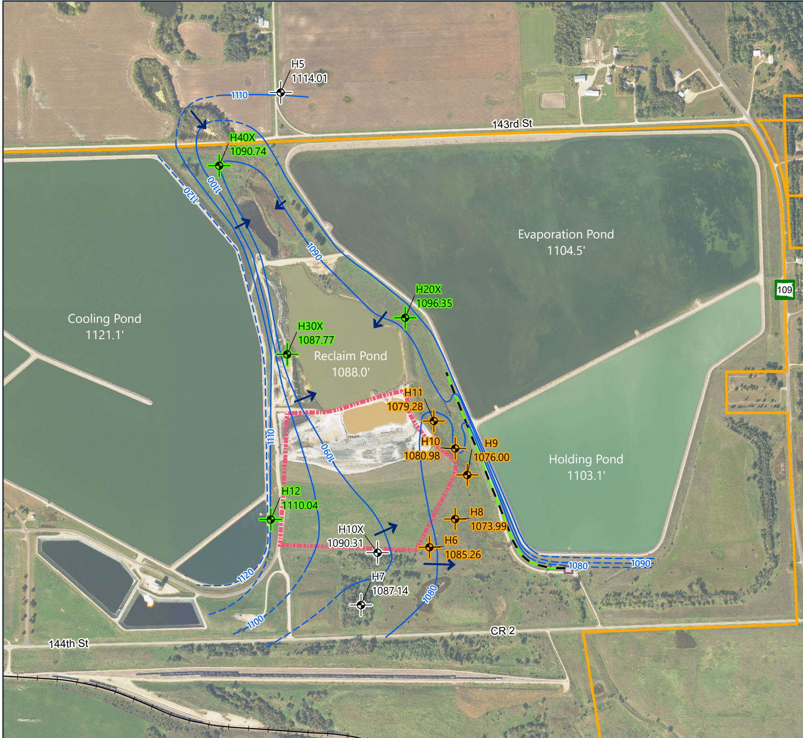
Groundwater Elevation Contours Fall 2025 Big Stone Plant Big Stone City, SD Otter Tail Power Company FIGURE 3
